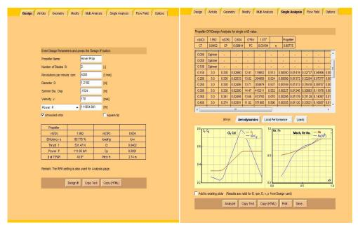
Figure 18 - Input screen for JavaProp
