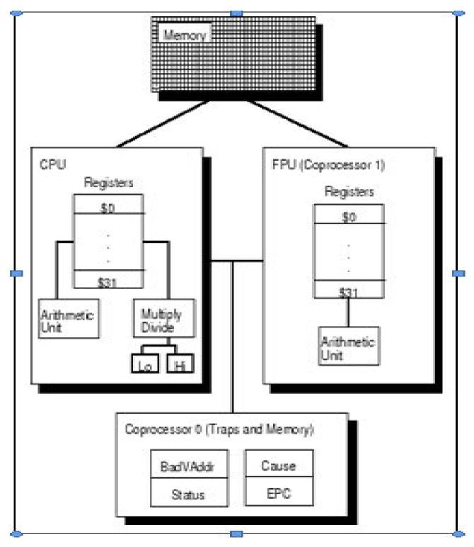
Fig.1. Block Diagram of MIPS R2000
