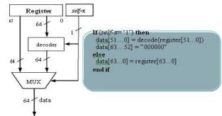
Fig. 5. Microarchitectural support for reading a register value.
