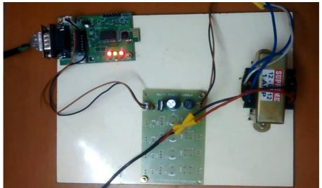
Fig 15 Receiver side of the smart dust mote
