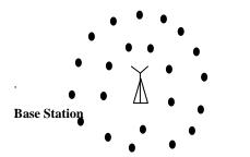
Fig 1.An example of wireless sensor nodes in a network sensing temperature in a particular area and reporting to base station.
