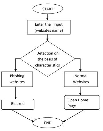
Figure 2: Phishing detection program flow chart
