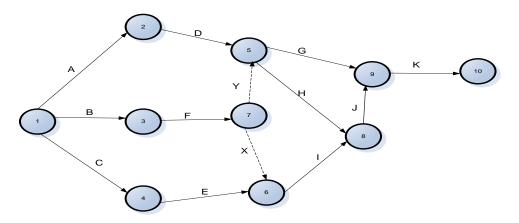
Figure 2. A simple Pert Network of the Space Module Assembly
