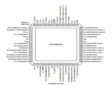
Figure 1: Pin diagram LPC 2138.
