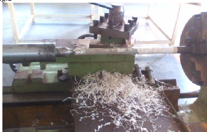
Fig. 2 Composite material taken out by turning operation
