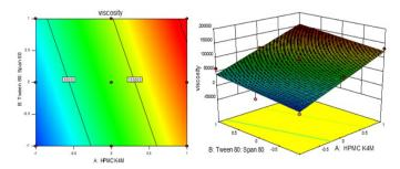
**Figure 8.** (A) Contour plot and (B) Response surface plot showing relationship in between viscosity of emulgel and polymer concentration.
