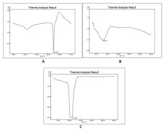
Figure 3. DSC Thermogram of pure drug A. Norfloxacin, B. HPMC K4M and C. Emulgel.
