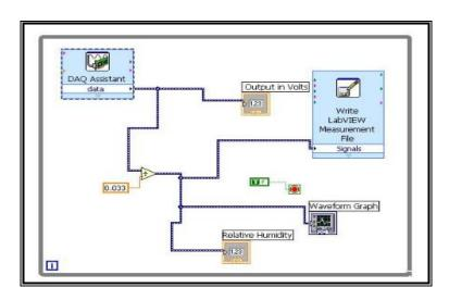
Fig 2(a): VI Block diagram of Humidity Measurement
