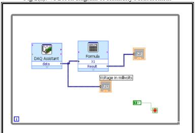
Fig 2(b): VI Block Diagram of Temperature Measurement
