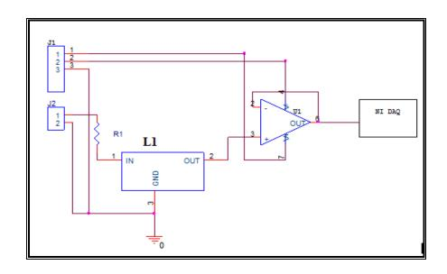
Fig 3: Circuit diagram of Clinical thermometer using LM 35
