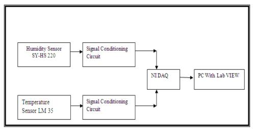
Fig 1: Functional Block Diagram of Humidity and Temperature Measurement System
