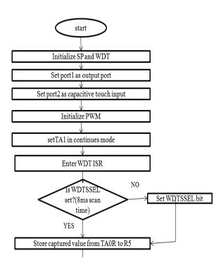
Figure 5: Flowchart of control unit.
