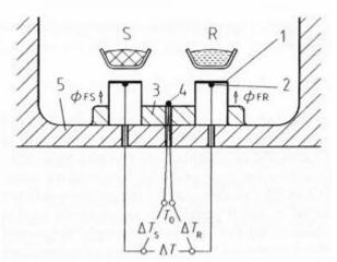
Figure 4: The turret type measuring system HF-DSC [7]
