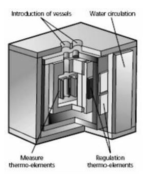
Figure 5: The heat flux Micro differential DSC
