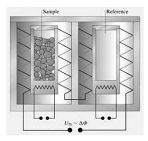
Figure 3: The heat flux DSC with a cylinder- type measuring System (Calvet)<sup>[10]</sup>
