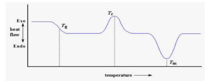
The crystallization peak and the melting dip will only show up for polymers that can form crystals and melts. Completely amorphous polymers won't show any crystallization, or any melting either. But polymers with both crystalline and amorphous domains will show all the features for the glass transition, there is no dip, and there's no peak, either. This is because there is no latent heat given off, or absorbed, by the polymer during the glass transition.
