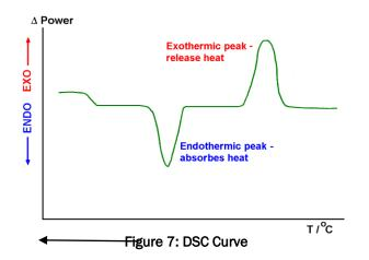
The result of a DSC experiment is a curve of heat fluxversus temperature or versus time. This curve can be used to calculate enthalpies of transitions, which is done by integrating the peak corresponding to a given transition. The enthalpy of transition can be expressed using equation:
