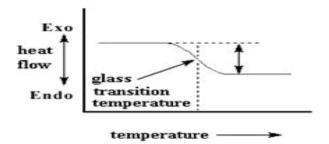
This means there is more heat flow. There is an increase in the heat capacity of the polymer. This happens because the polymer has just gone through the glass transition (It is a reversible transition in amorphous material from a hard, brittle state into molten rubber like state).Because of this change in heat capacity that occurs at the glass transition, we can use DSC to measure a polymer's glass transition temperature.
