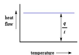
The heat flow is heat (q) supplied per unit time (t), whereas, The heating rate is temperature increase ( $\Delta T$ ) per unit time (t),
