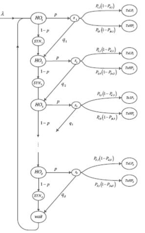
Figure 4. The Markov process of modified p-persistent access (MPPA) scheme for each secondary user's sensing- transmission process.
