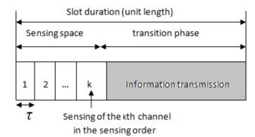
Fig.2. slot structure(when a secondary user stops after its *k*th sensing) If the two users simultaneously decide to stop at the same channel, one of the following three contention level strategy will apply.1)FAIL\_THEN\_CONTINUE, 2)FAIL\_THEN
