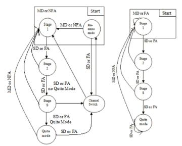
Fig. .3. Schematic representation of the considered multichannel multistage spectrum sensing algorithms. (a)Single narrowband radio case and (b) parallel narrowband radios case. MD: misdetection, SD: successful detection, FA: false alarm, NFA: no false alarm; dashed line: algorithms involving quiet mode; dotted line: algorithms involving presenting mode. Note that for brevity, we did not mark the transition to and from the idle stage if there are no frames to transmit.
