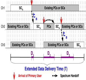
Fig. 1. An example of transmission process for the secondary connection SCA, where ts is the channel switching time, T is the extended data delivery time of SCA, and Di is the handoff delay of the ith interruption. The gray areas indicate that the channels are occupied by the existing primary connections (PCs) or the other secondary users' connections (SCs). Because SCA is interrupted three times in total, the overall data connection is divided into four segments.
