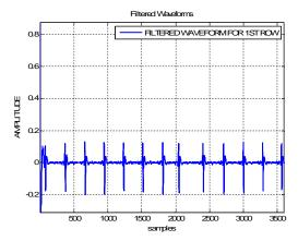
Figure 5 Filtered ecg for 1st row
