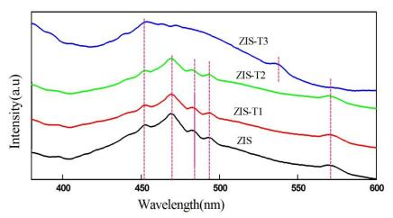
Fig.9 PL Spectrum of the of the as-deposited and annealed ZIS film
