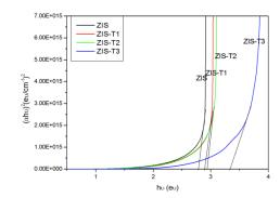
Fig.5 Absorption coefficient of the as-deposited and annealed ZIS film deposited and annealed ZIS film
