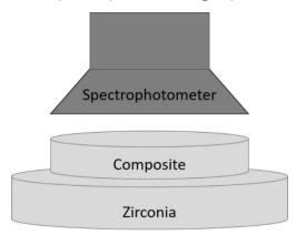
Figure 2. Diagram of the tested specimen and color measurement.
