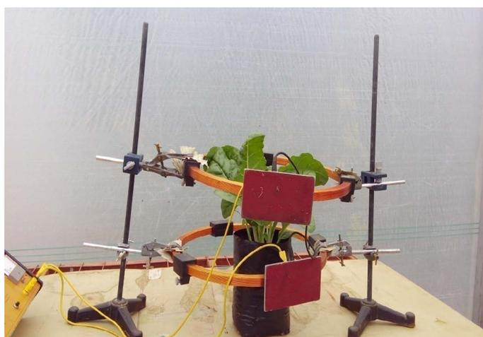
**Figure 1.** The schematic representation of the magnetic flux density exposure designs showing the arrangement of Helmholtz coils.
