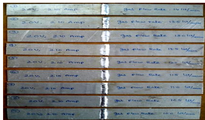
Fig .3. Welded specimens
