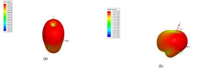
Fig.4.Directivity of a) Central feed monopole b) Feed located monopole
