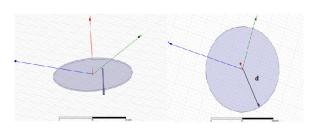
Fig.2. a)Side view b) Top view of a feed located wire monopole antenna geometry Where d is distance of antenna which is placed 40,40 mm from origin in x,y direction respectively.Fig2: - shows the geometry of a monopole placed at a distance of(40,40) mm from origin.
