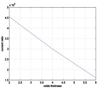
Fig 6:  $I_{on}/I_{off}$  current ratio vs. oxide thickness with same conditions as in fig 1
