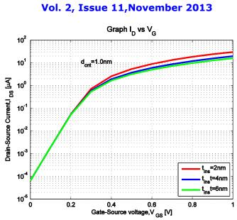
Fig. 2 Effect of insulator thickness on I<sub>DS</sub> vs. V<sub>GS</sub> in logarithmic scale. To obtain the I<sub>off</sub>, the curve is shown in logarithmic scale.
