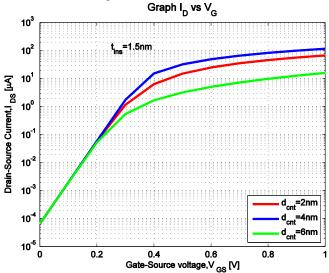
Fig4: Effect of diameter of CNT on  $I_{DS}$  vs.  $V_{GS}$  in logarithmic scale. To obtain the  $I_{off}$ , the curve is shown in logarithmic scale.
