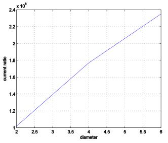
Fig 5: Ion/Ioff current ratio vs. diameter of CNT with same conditions as in fig 1
