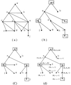
Fig. 1 An illustration of our algorithm. (a) Shows the example network. (b) Shows the BFS tree, (c) Shows the broadcast tree, (d) shows the transmission schedule.
