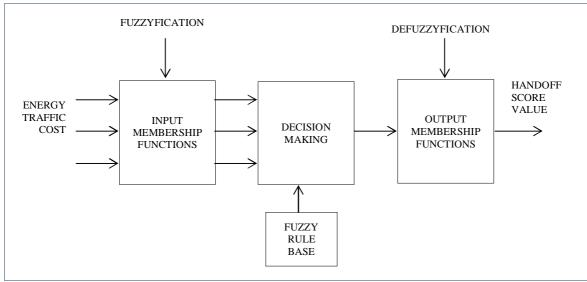
Fig 2. Block diagram of Fuzzy Logic System
