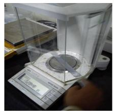
Figure 8: Weight apparatus to measure electrode weight
