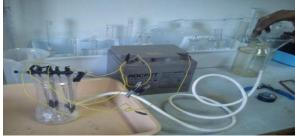
Fig1. Mono polar electro coagulation setup
