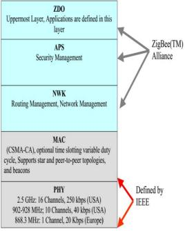
Figure 2.ZigBee(TM) Stack
