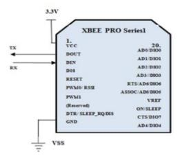
Figure 4: Schematic diagram for XBEE
