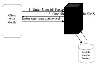
Fig. 2. One Time Pad Password Authentication.
