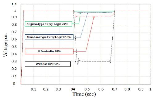
Fig. 12 (a) Single-Phase Comparision of Sugeno-Type Fuzzy Logic, Mamdani-Type Fuzzy Logic, PI Controller, and Without DVR
