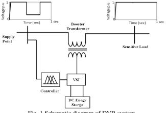
Fig. 1 Schematic diagram of DVR system
