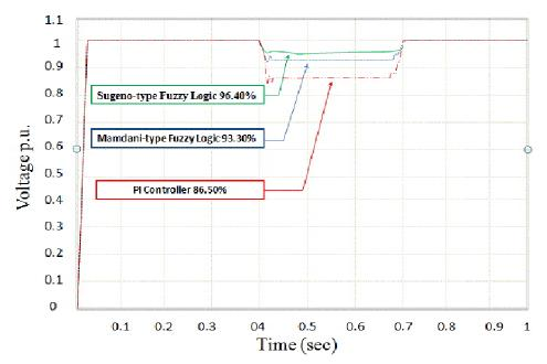
Fig. 13 (b) Two-Phase Comparision of Sugeno-Type Fuzzy Logic, Mamdani-Type Fuzzy Logic, and PI Controller
