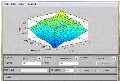
Fig. 10 Surface View Using Mamdani-type Fuzzy Logic Algorithm
