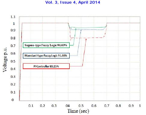
Fig. 14 (c) Three-Phase Comparision of Sugeno-Type Fuzzy Logic, Mamdani-Type Fuzzy Logic, and PI Controller
