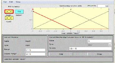
Fig. 4 Membership Function for Sugeno-type Fuzzy Logic Input Variable
