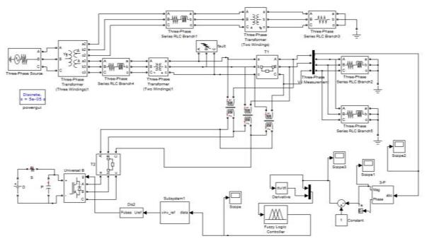
Fig. 9 Matlab/Simulink Power Circuit Model of DVR
