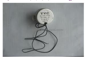
A synchronous electric motor is an <u>AC motor</u> in which the rotation rate of the shaft is synchronized with the <u>frequency</u> of the <u>AC</u> supply current; the rotation period is exactly equal to an integral number of AC cycles. Synchronous motors contain <u>electromagnets</u> on the <u>stator</u> of the motor that create a <u>magnetic field</u> which rotates in time with the oscillations of the line current. The <u>rotor</u> turns in step with this field, at the same rate.
