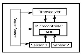
Fig.1 Block diagram of Sensor node
