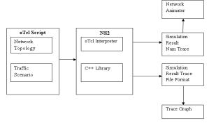
Fig. 8 Block Diagram of Ns2
