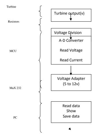
Figure 4.2: Flow Chart for the Data Acquisition Board
