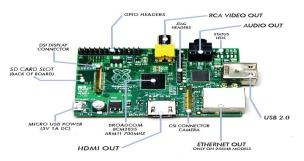
Figure2.Raspberry board with its components
