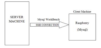
Figure5. Connection with MySQL in client machine through SSH
