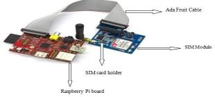
Figure6.SIM 900 GSM/GPRS module connected with Raspberry Pi
