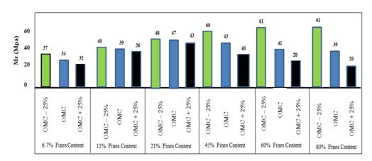
Figure 5. Variation of Mr values due to fluctuation of moisture and fines content.
