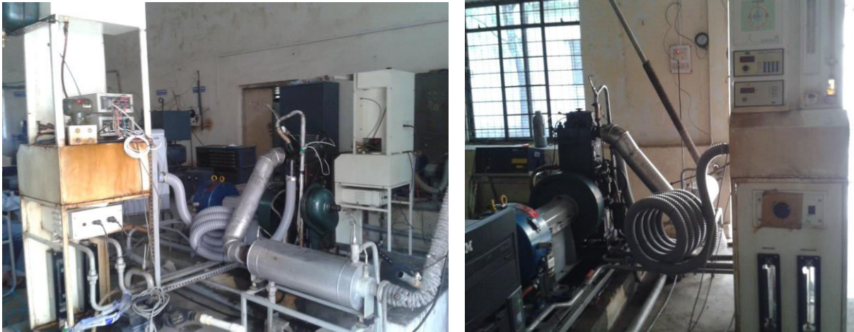
Fig. 1 Experimental set up with 3 and 5 turns in pipe connecting inlet manifold and air chamber
