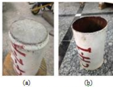
Plate (11) Shows deformation of circular unstiffened columns (a) Filled concrete (A) column (b) Hollow column
