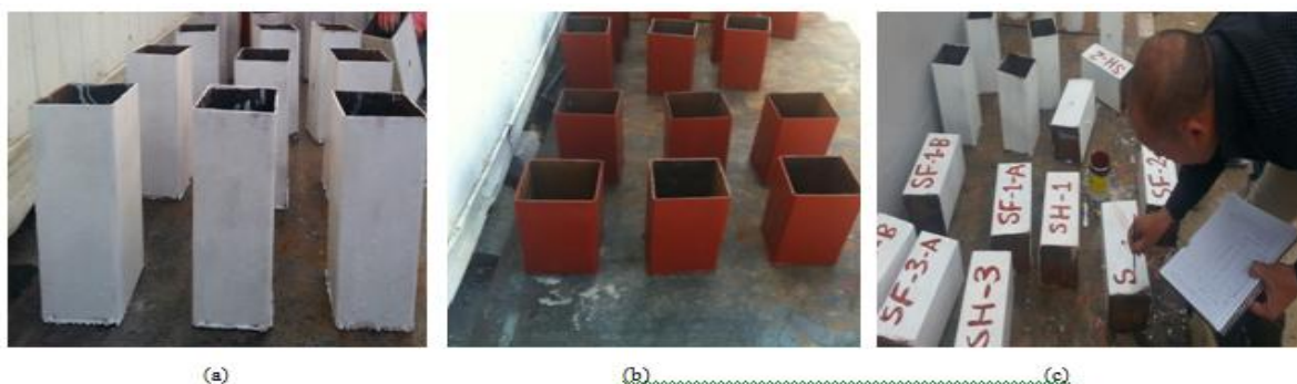
Plate (1) Unstiffened square (CFST) stub columns (a) White painting (b) Red painting (c) Writing symbols
