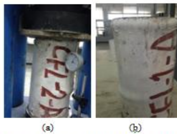
Plate (13) Shows deformations of reinforced circular (CFST) columns (a) 4mm tube thickness (b) 3mm tube thickness
