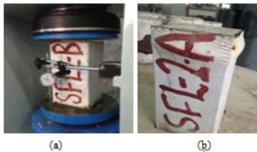
Plate (10) Shows deformations of reinforced square (CFST) columns (a) Reinforced filled concrete (B) (b) Reinforced filled concrete (A)
