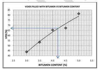
Figure 2:- Voids Filled with Bitumen V/s. Bitumen Content
