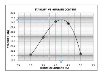
Figure 3:- Stability V/s. Bitumen Content
