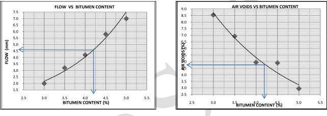
Figure 5:- Flow V/s. Bitumen Content
