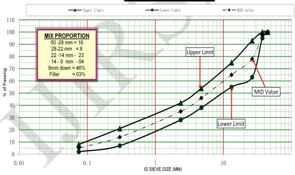
Figure 1:- Graph of DBM Gradation Curve
