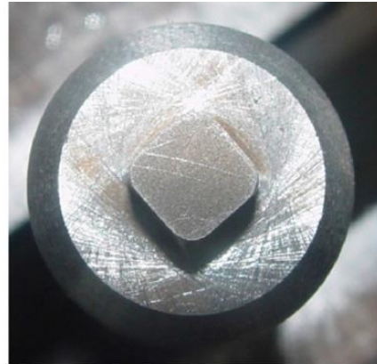
Fig.2d. Square Pin Profile Tool
