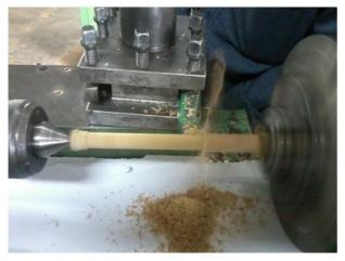
Fig.4 Lantana Camara stem turned in lathe The powders are collected from the tray under the chuck. Fine powders are obtained by crushing the
