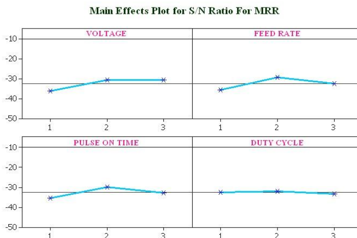
Fig. 5 Main Effects Plot for (S/N Ratio) of MRR in PECM
