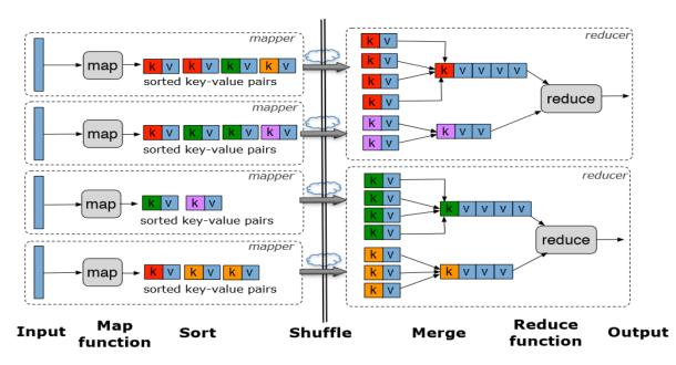
Fig. 3. Map Reduce Data Flow Diagram
