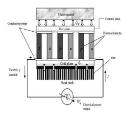
Fig.4 principle of TEG
