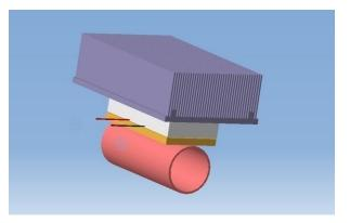
Fig.3 TEG assembly model
