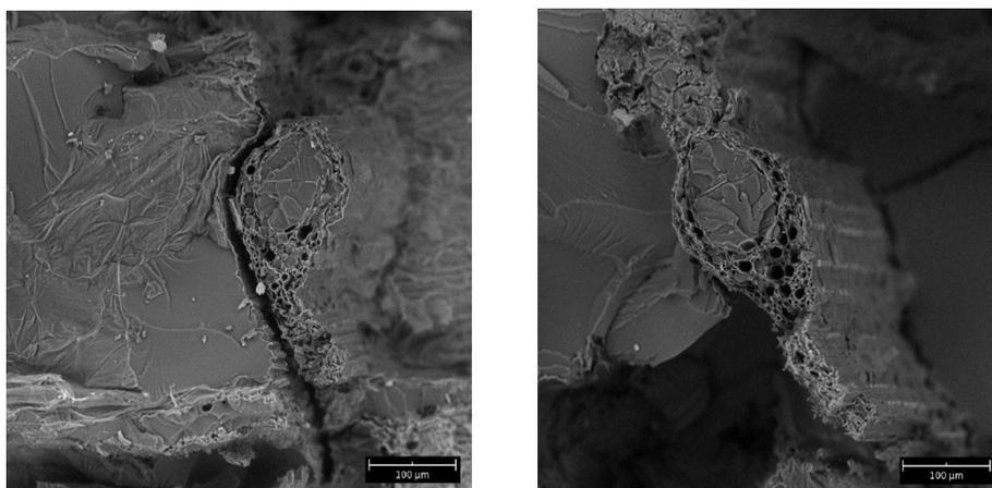
**Figure 3.** SEM Micrographs of fractured surface of the alkali treated cellulose fiber Composite fiber-matrix bonding (500x Magnification) a) Crack Formation b) Unfilled Holes of the Fiber.
