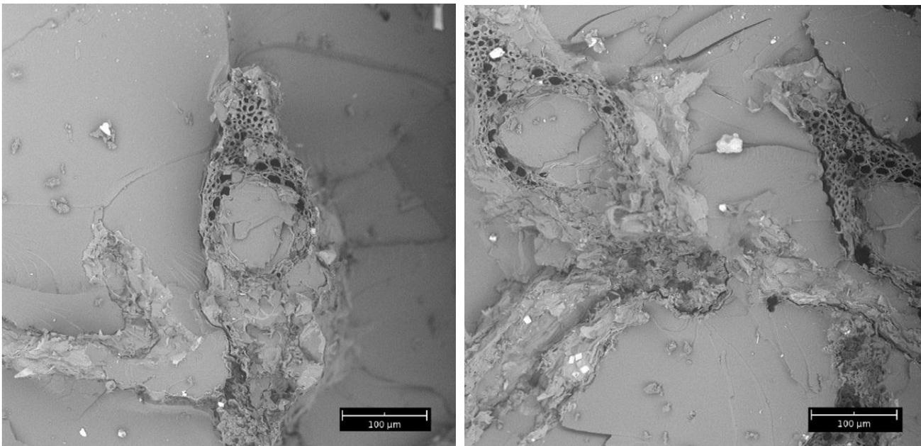
**Figure 4.** Scanning Electron Micrographs of the Fractured Surface of the Combined Alkali-Bleach Treated Mengkuang Cellulose Fiber Composite (500x Magnification).
