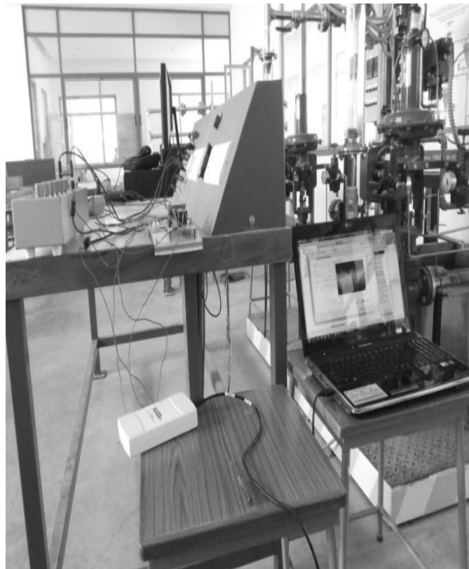
Figure 2. The experimental setup of pneumatic actuator fault diagnosis
