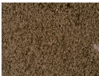
Figure 8. Feralgine powder (picture making by stereomicroscopy Wild Heerbrugg Makroskop M420 linked to an OPTIKAM MICROSCOPY DIGITAL USB CAMERA) [16].
