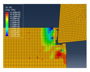
Figure 5 Shear Force in X direction
