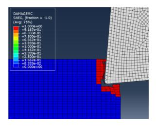
Figure 4 Matrix damage plot
