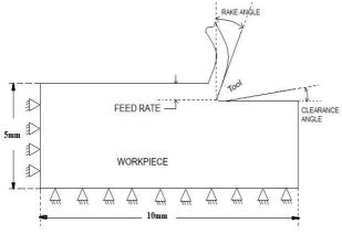
Figure 1 Model geometry and boundary conditions
