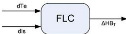
Fig. 7. Block diagram of the proposed FLC for hysteresis band adaptation.
