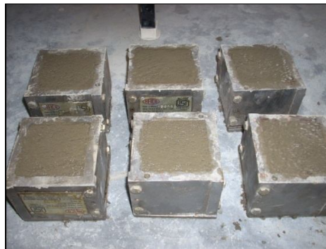
Fig. (4) Casting of control specimens
