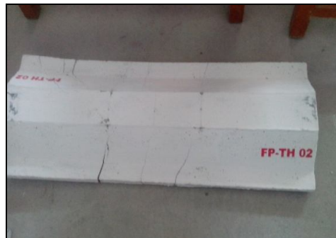
Fig. (14) Crack pattern (FP-TH 02)
