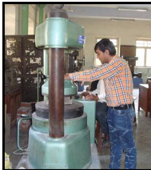
Fig 6: Compressive strength testing
