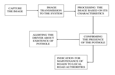
Fig.: Functional Block Diagram of The FPGA Based Intelligent Potholes Detection System
