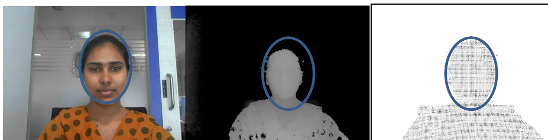
Fig 2: Misalignment of object in RGB (left) and Depth (Middle) images (Observe -Scaled down face in depth image) and Depth-Mask (right) image in align with RGB image.
