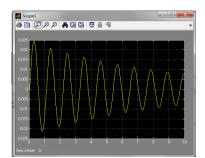
Figure 7: Rotor speed deviation for 5% change in mechanical power input with Constant Field Excitation only.
