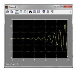
Figure 9: Rotor speed deviation for 5% change in mechanical power input with AVR and K5 Negative.
