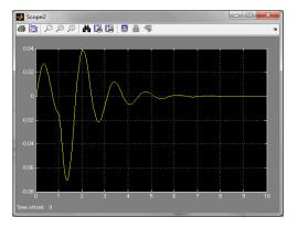
Figure 8: Rotor speed deviation for 5% change in mechanical power input with AVR and K5 Positive.
