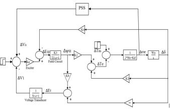
Figure 4: PSS in State-Space model of SMIB system.
